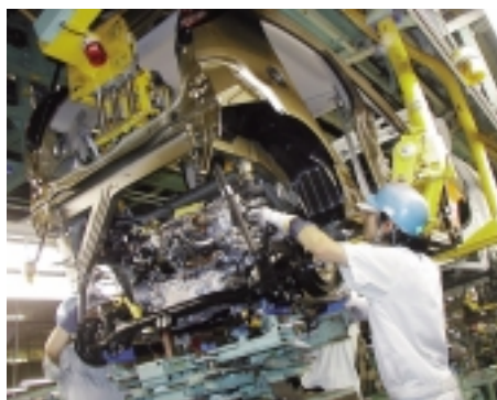
Fitting the rear engine in the "i"
